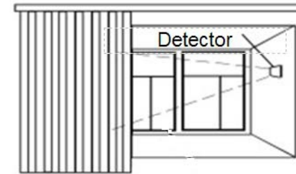
Fig.5 Detector mount between window and curtains (louvers)
